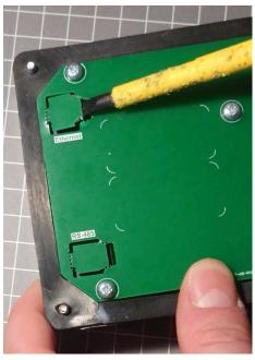
2. Connect the remote equipment to the RJ45 port using a **double insulated** Ethernet cable (e.g. Clipsal 5005C305B).
